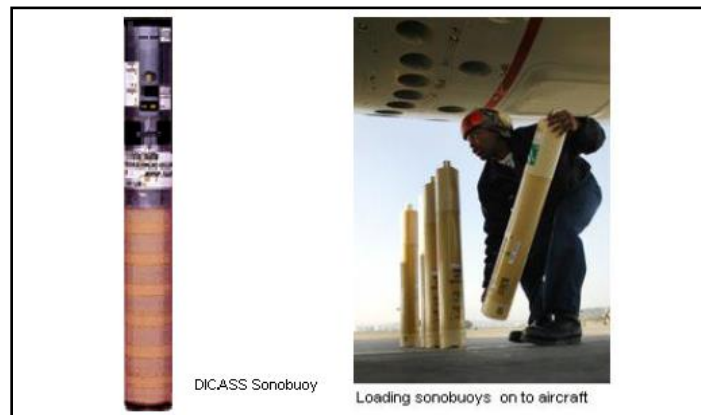
Figure A.1-4: Sonobuoy (e.g., AN/SSQ-62)
